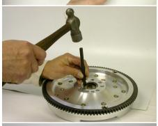
IF THIS PLATE DOES NOT FIT THE ALUMINUM FLYWHEEL, STOP INSTALLATION AND CALL THE FIDANZA TECH LINE OR EMAIL. The center hole measures 38mm from the engine side on 193461. The 193361 measures 28mm and does not require the center plate and will not interchange with 193461.
