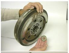
If this plate is not installed in the aluminum flywheel, there will be no center hole for clutch alignment tool.
