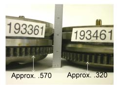
The ring gear placement is different between the two flywheels. The ring gear placement on a 193461 is closer to the block than the 193361. The ring gear placement MUST be verified before installation.
